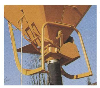
The patented TU gate mechanism is the bench mark for all column skips. This gate is fitted as standard to all TU/TUC skips and can be fitted with numerous accessories including quick release fittings for differing diameters of discharge hose, adjustable discharge funnel and chutes.
